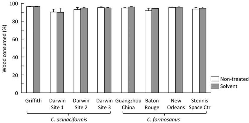
Fig. 3. Mean percentage wood consumption of nontreated and solvent-treated control specimens after exposure to *C. acinaciformis* and *C. formosanus* at field test sites in Australia, China, and the United States.
