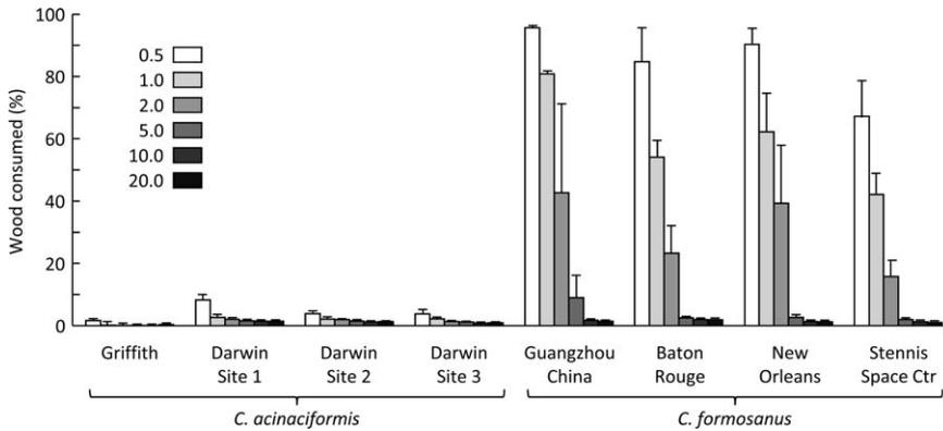
Fig. 5. Mean percentage wood consumption of bifenthrin-treated specimens after exposure to *C. acinaciformis* and *C. formosanus* at field test sites in Australia, China, and the United States. Bifenthrin retentions ( $\text{g AI/m}^3$ ) indicated in the legend.
