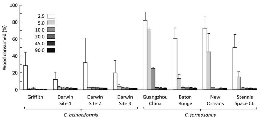
Fig. 6. Mean percentage wood consumption of permethrin-treated specimens after exposure to *C. acinaciformis* and *C. formosanus* at field test sites in Australia, China, and the United States. Permethrin retentions ( $\text{g AI/m}^3$ ) indicated in the legend.
