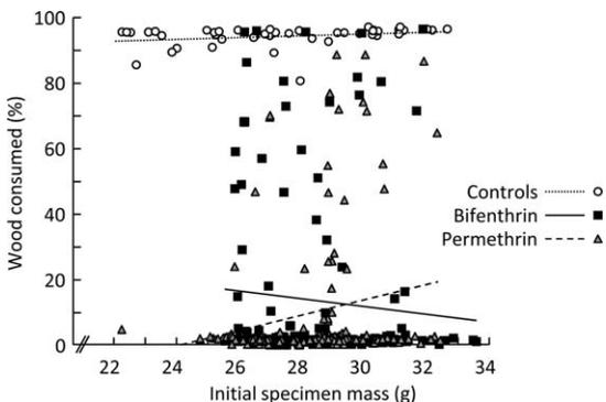
Fig. 4. Percentage wood consumption plotted against initial mass for each test specimen exposed to *C. acinaciformis* and *C. formosanus*. The regression equations for percentage wood consumed against initial mass of specimen are: controls,  $y = 0.867 + 0.003x$  ( $r^2 = 0.079; F = 3.592; df = 1,42; P = 0.065$ ); bifenthrin,  $y = 0.468 - 0.011x$  ( $r^2 = 0.007; F = 0.877; df = 1,130; P = 0.351$ ); and permethrin,  $y = -0.511 + 0.022x$  ( $r^2 = 0.046; F = 6.238; df = 1,130; P = 0.014$ ).
