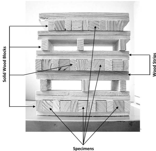
Fig. 2. Arrangement of pyrethroid-, solvent-, and nontreated specimens ( $25 \times 25 \times 100$  mm) in three parallel horizontal tiers, separated by two double-layer wood strips (each strip  $10 \times 45 \times 215$  mm) between tiers, with solid wood blocks ( $15 \times 25 \times 100$  mm) of *P. radiata* sapwood adjacent to specimens within each exposure container.
